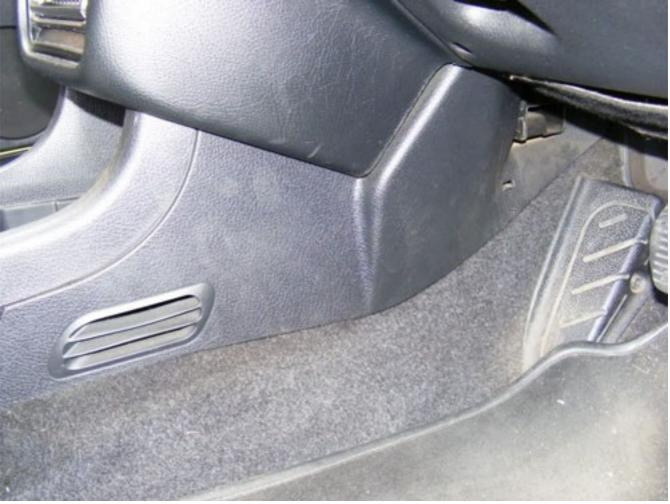
Put the torx20 screw back in under the drivers footwell:
