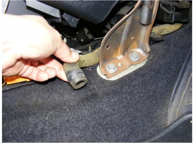
Refit the lower vent tube. Due to the metal bracket in the way & the fact it has a slope at the upper end, it's tricky to get it to fit right. It actually fits fully over the bit behind the dashboard. You'll know it's fitted right when the flat plastic tab (circled in red) slots into the centre console unit, if it won't go in, then it's not properly over the heater unit:
