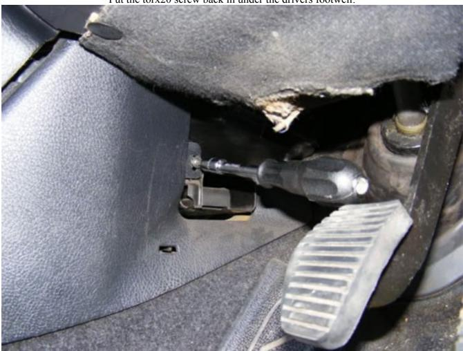
Refit the other torx20 screw inside the console:
